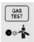
By pressing the gas-feed test key, you can make the shielding gas flow without starting the power source or the wire feed. This enables the measuring of the gas flow with an external measuring device.
